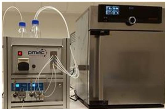
The **PMAC** System provides an accurate, reproducible and rapid method for selecting and quantifying the most effective means of controlling scale deposition under dynamic conditions. PMAC scale rigs are being used by many laboratories around the world to provide accurate and repeatable results and seen as the Industry Standard by the leading Major Oilfield Chemical Companies.
